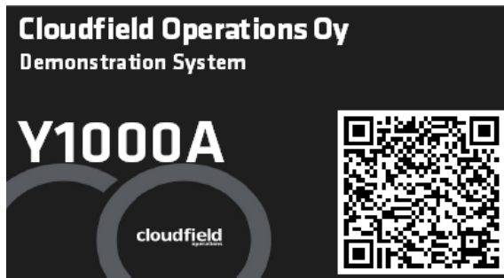
Figure 1: Example sticker with machine understandable reference designator of the actuator position
